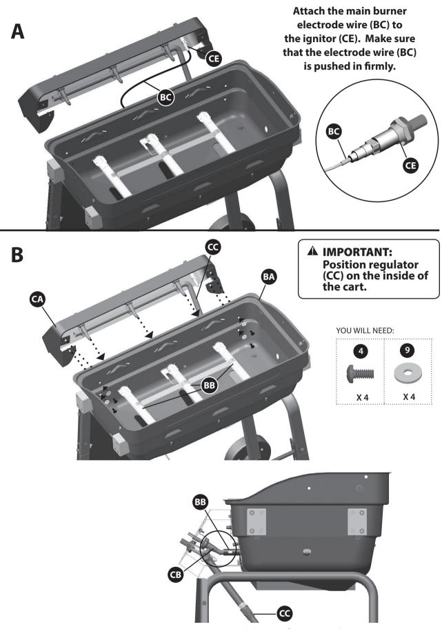
Position Valves (CB) into Burner Tubes (BB) before assembling.
