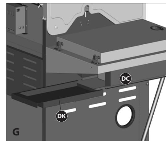
g. Insert the infrared grease tray (DK) into the bottom of the infrared support frame (DC).
