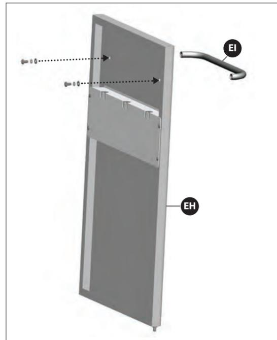
Assemble the Door Handle (EI) to the Left and Right Door Assembly (EG and EH).
