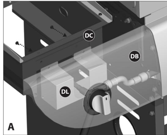
a. Assemble the venturi wind shield (DL) to the infrared support frame (DC).
