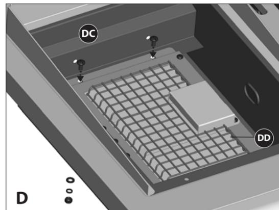
d. Assemble the infrared side burner (DD) to the infrared support frame (DC), at the two points indicated in figure D.
