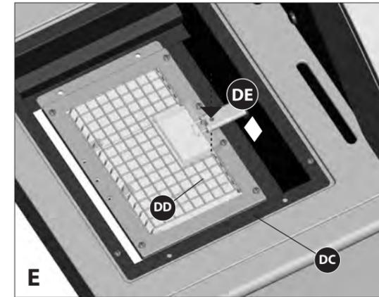
e. Feed the infrared electrode (DE) from underneath the infrared side burner (DD), through the small opening on the right side of the infrared support frame (DC). Align and assemble the electrode using the self tapping screw provided, as shown in figure E.
