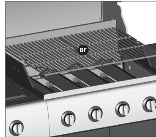
Place the cooking grates (BF) into the burner box (BA).
