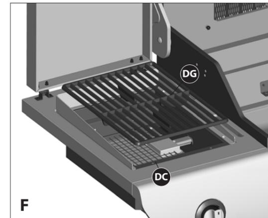
f. Position the cooking grate (DG) on the infrared support frame (DC).
