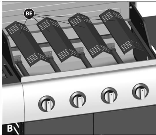
b. Position the Flame Tamers (BE) into the Burner Box (BA).
