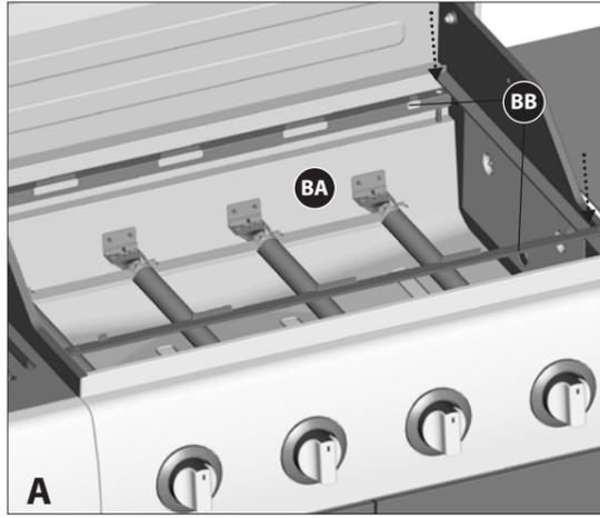
a. Position the Flame Tamer support braces (BB) over the Burner Box support pins (BA) as shown.
