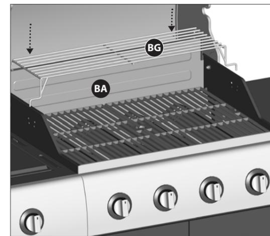
Insert the two small positioning rods of the warming rack (BG) into the rear panel of the burner box (BA).
