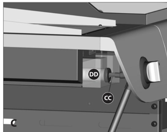
c. Make sure that the infrared burner (DD) engages the side burner valve (CC), as shown in figure C.
