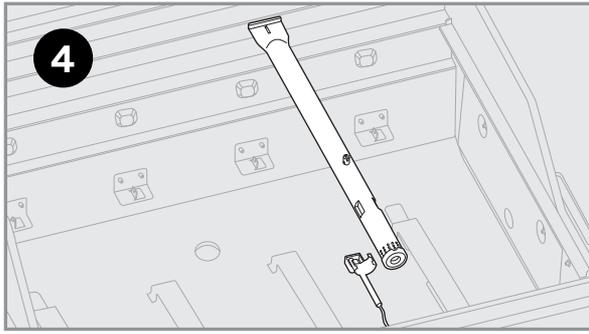
3. When installing your new burners, start with the lighting burner. Attach the electrode clip to the underside of the burner. **Figure 4**
